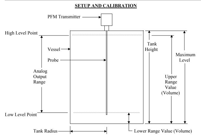
Determine the Maximum Level. This is the highest point that can possibly be measured. This is usually, but not always, the same as the tank height. Fill in the value below.
